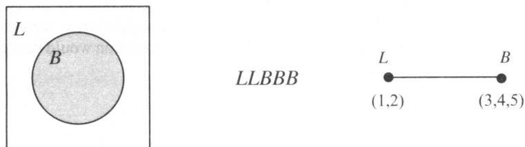
Figure 10.39: Optimal segmentation and interpretation: interpretation, corresponding code string, and region adjacency graph.
